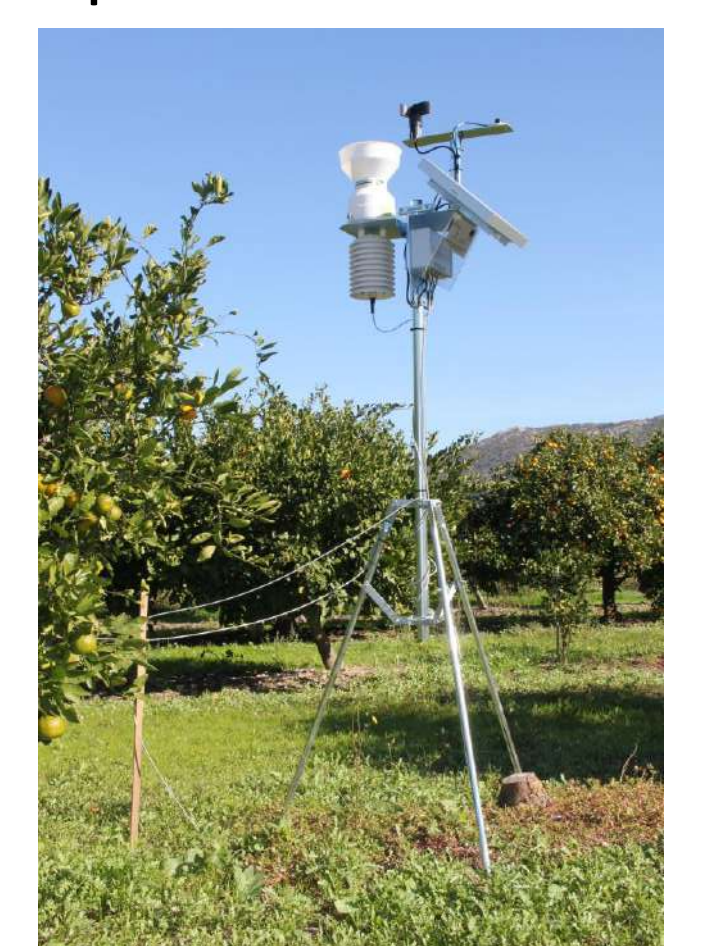
Automatic weather station at SML1
